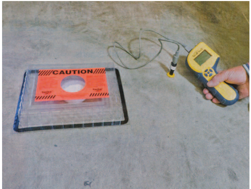
The calcium chloride dome test and the in situ relative humidity test provide fundamentally different information on a floor's moisture condition.
